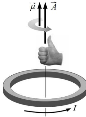
Figure 7.3: Direction of the magnetic dipole moment of the current loop.
