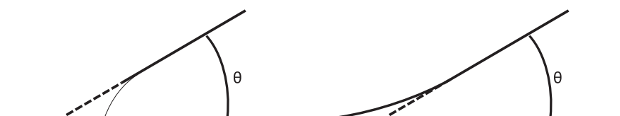
Fig. 10. Liquid/vapor interface deviates from the apparent contact angle near the three-phase contact line due to the presence or absence of long and short range molecular interactions.
